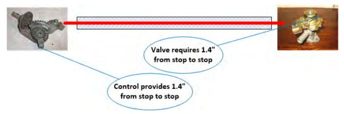
The heater control system we use was originally designed in the early 1950's for the MGA. If you picture a right hand drive MGA, the control would be perhaps 18" away from the valve; a straight shot through the firewall. Fast forward to the North American 1968 – 1974 MGB and we have the worst possible evolution. The control now sits on the left side of
