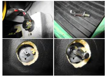
Inside the cockpit, you can just mount the potentiometer housing under the dash and ignore the original dial. I decided I wanted the control to be in the stock position and that I wanted to use a stock knob. The potentiometer supplied is too short to reach through the dash so I grafted on the shaft that I sawed off from a stock control. This let's me use the regular knob and keeps the dash looking normal. (photos - above right)
