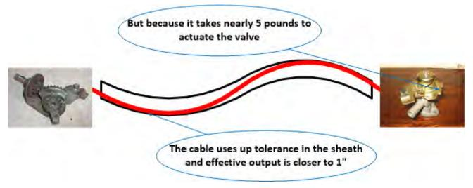
The length, the curve and the force together mean that the cable no longer emerges at the valve end with the same distance that you move it at the control. Your 1.4" has become 1". Practically speaking this means that when you setup your heater valve, you must choose between having it fully open **or** fully closed. It is unlikely that you can have both. Freeze in the morning, or heat blowing on your feet when you're driving on a hot sunny day.
