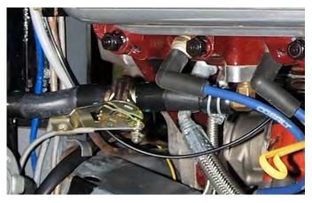
This valve is still era-appropriate with a zinc plating and simple mechanics. It doesn't look out of place under the hood and uses the stock control and cable. It comes with the sheath hold down and best of all it requires less than one pound of force to open and close in less than 1.3" of throw. This means that despite the cable length and turns, the valve fully operates.
