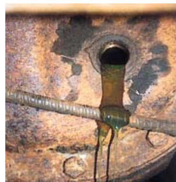
4) The axle is filled to the correct level when the oil reaches the filler neck.
