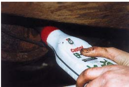
3) Undo the refill plug which is located about halfway up the back of the axle cover and fill the back axle with the recommended oil.
