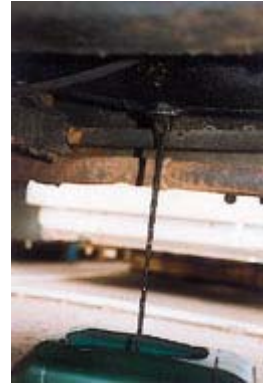
6) Carefully remove the drain plug by hand and drain the old gearbox oil into a suitable waste oil vessel. This one was made from an old plastic oil container with a hole cut out of the side.
