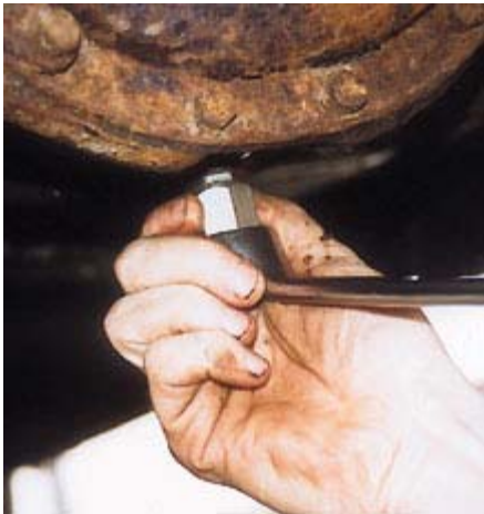
1) Undo the drain plug at the bottom of the axle casing using a square drive socket.
