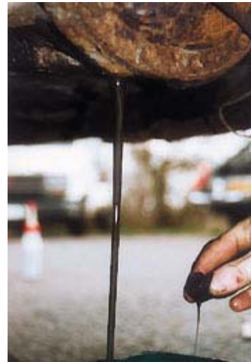
2) Drain the old back axle oil into a suitable waste oil container. Once the axle casing has completely drained replace the plug.
