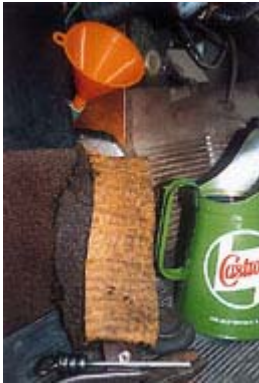
9) Using a funnel connected to about five inches of garden hose you can make an effective refill system.
