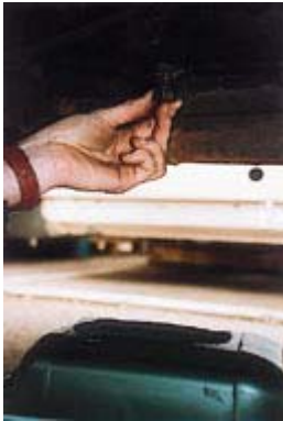
7) Allow sufficient time for the oil to drain completely from the gearbox. Once you are satisfied that all the oil has run out, then refit the drain plug.
