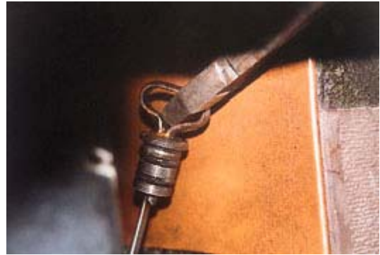
8) If you have an earlier model MGB the gearbox will be filled by a combined dipstick/filler plug which is situated under a rubber plug in the transmission tunnel and reached from within the cockpit. It can be very difficult to remove this dipstick, it sometimes helps if you have a length of cord looped through the dipstick handle. Alternatively you can usually pull it out with a pair of pliers.
