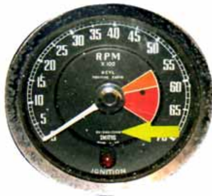
1. Face of an RVI series tachometer showing where to read the tachometer identity
