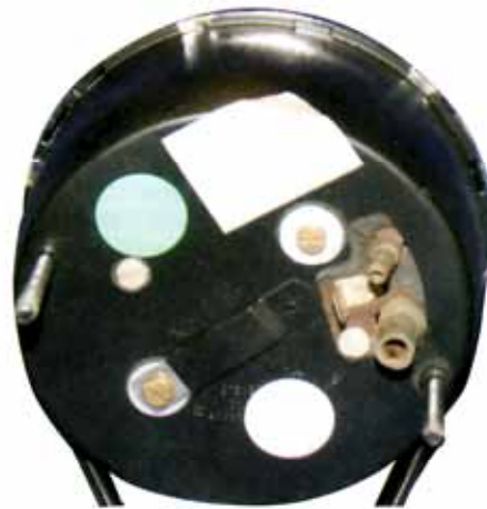
3. Rear of later RVI series tachometer with internal sensor loop and a male and female external bullet connectors, plus the separate spade connection for tachometer power feed
