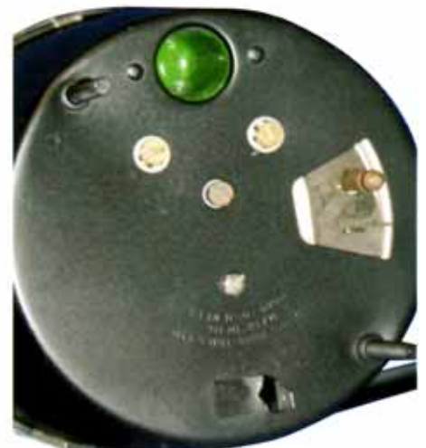
4. Rear of an RVC tachometer showing just a single male bullet connection and separate spade connection for the tachometer power feed. This particular tachometer has a separate earth spade connection whilst most simply earth through the fixings between tachometer and dashboard
