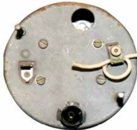
2. Rear of early RVI type tachometer with the external sensor loop and separate spade connection for tachometer power
